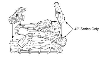
Figure 50 - Installing Log No. 6 and Log No. 7
